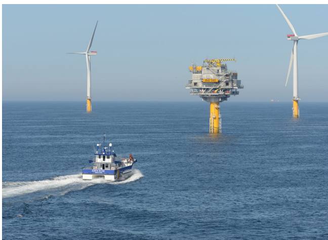
Figure 1. Crew transfer vessel (CTV) carrying crew and equipment to an offshore wind farm.
