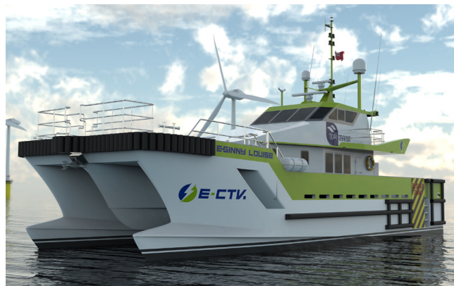
Figure 3. Render of e-Ginny, the world’s first diesel-to-electric retrofit CTV.
